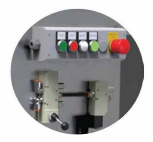
The control panel allows the operator to control the time, temperature and airflow of the thermal dryer.
