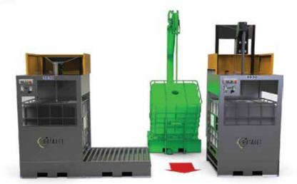
To increase drying capacity an additional RJ-TVS Tipping Vac station is retrofitted into the line. This addition will allow more IBCs/hour to be processed.
