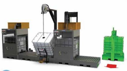
To ensure the integrity of the IBCs, a RJ-PT Pressure Testing station is fitted after drying.
